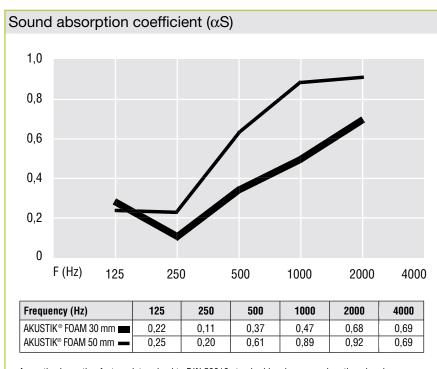
Acoustic absorption factors determined to DIN 52212 standard in a large reverberation chamber
