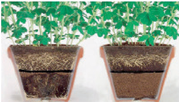
Bituminous Waterproofing membrane without and with antiroot additive Preventol B2.
