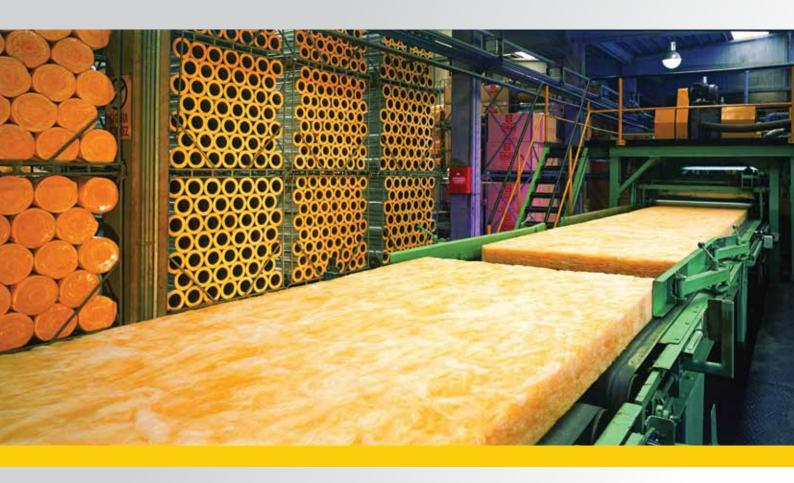
Glass wool is made from an inorganic raw material, which is obtained domestically. It is produced through heating row material at 1200°C - 1250°C and transforming it into fibres. It can be manufactured in the forms of blanket, board or pipe in different size and with different technical properties, with different facing materials according to the intented use and the place of use. It is used for thermal insulation, sound insulation, acoustic comfort as well as fire safety.
